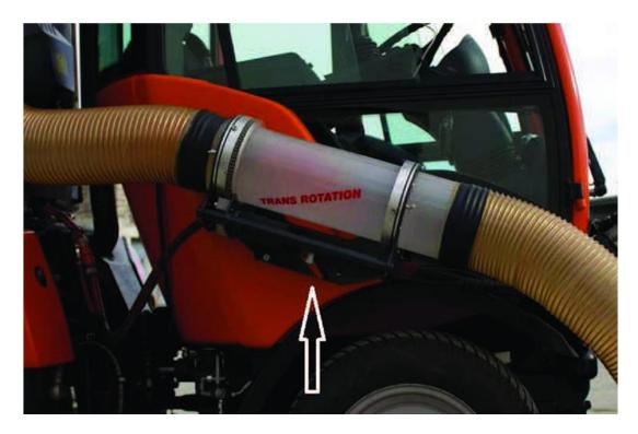
The length of the suction hose must be adjusted during the initial installation and again after the initial break-in period. Adjust the rear portion of the hose while the tractor's steering at its maximum left turn. With the sweeper unit lowered, stretch the front portion of the hose slightly and adjust it as necessary. Check and adjust the length of the hose periodically as prolonged use may stretch it slightly.
