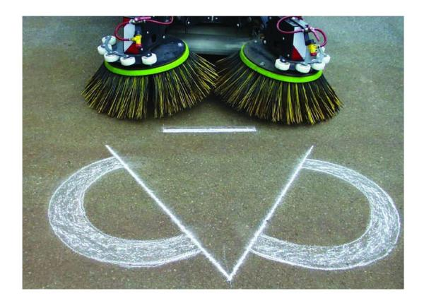
The forward and outward tilt ensures that the brushes sweep dirt and debris towards the suction mouth.
