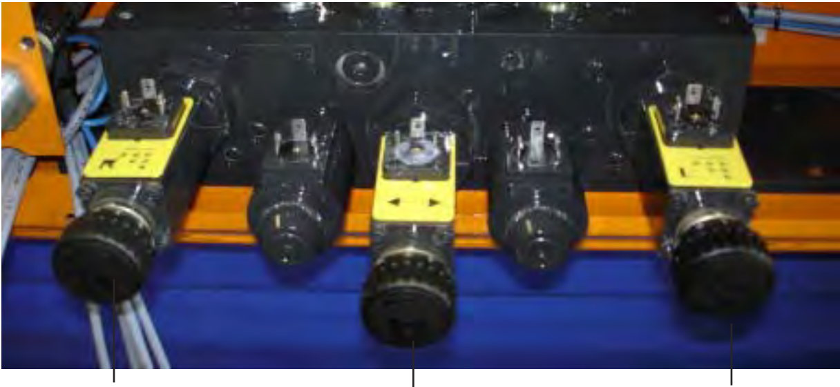
Hand wheel right-hand conveyor screw Hand wheel for emergency operation of spreading disc Hand wheel for left-hand conveyor screw
