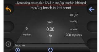
Repeat this procedure for all spreading materials available in the spreader. Left and right screw respectively.
