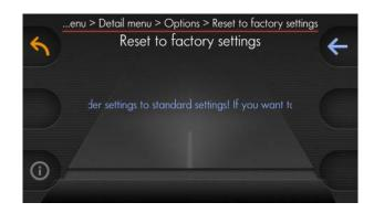
Press middle turning knob to reset the control system to factory settings
