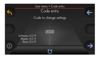
Hold down middle turning knob and turn until code entry "1000" is displayed
