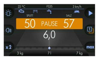
Turn left turning knob to change output rate of left chamber (Example: 58 g/m²)
