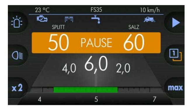
The adjustment of the spreading image may be converted to "Automatic spreading image".
