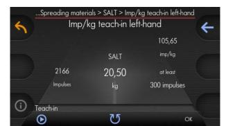
By turning the middle turning knob, correct the result with the difference
