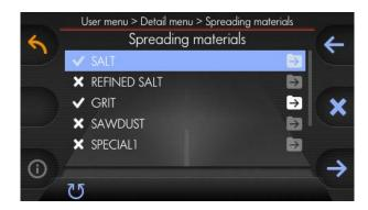
Choose corresponding spreading material (salt or refined salt)
