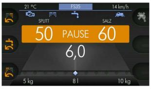
By turning the right or left turning knob, the spreading materials chosen before in the details menu, (see Chapter 7.9.1 "Setting of possible spreading materials", page 48) can be chosen and activated for the respective chamber.
