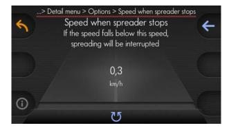
Setting of speed when the spreader should stop at the middle turning knob
